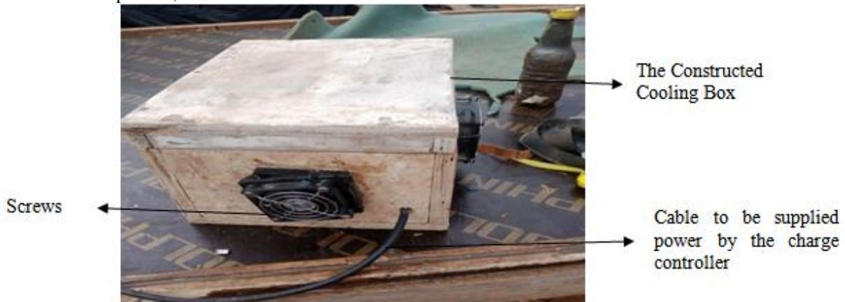
**Figure 8: Complete assembly of the constructed thermoelectric refrigerator.**
